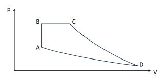
$$4T_A \ 2^{\gamma-1}V_A^{\gamma-1} = T_A V_D^{\gamma-1} \quad \rightarrow \quad 2^{\gamma+1}V_A^{\gamma-1} = V_D^{\gamma-1} \quad \rightarrow \quad V_D = 2^{\frac{\gamma+1}{\gamma-1}}V_A = 2^{\frac{5}{3}+1}V_A = 2^4 \ V_A = 16 \ V_A$$
