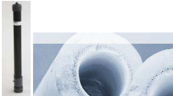
Figure 1: On the left: an example of hollow-fiber module. On the right: a magnified picture of a single hollow-fiber. Courtesy of Polymem - Toulouse, France.
