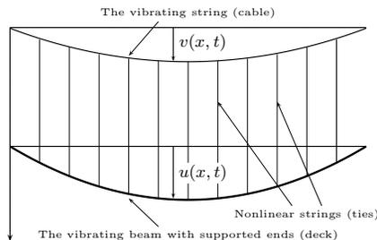
Figure 1: Center span hanged by main cable.
