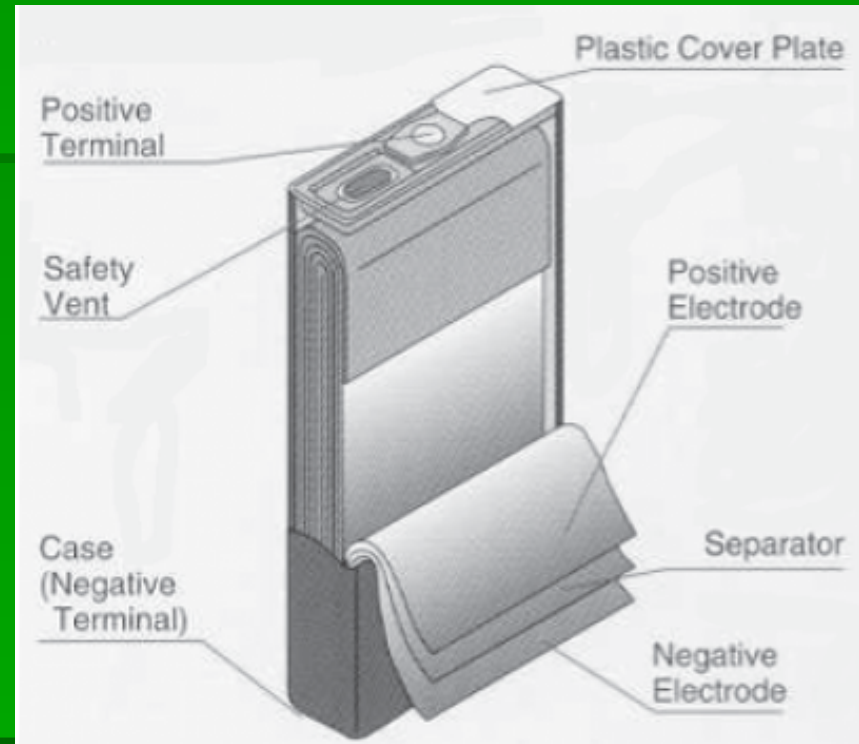
FIGURE Schematic drawing of a wound prismatic cell.
