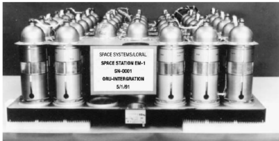
FIGURE International Space Station 81-Ah Ni-H 2 38-cell assembly.
