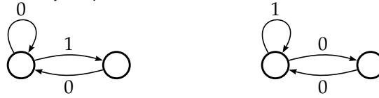
Figure 4: Finite automata for the G -shift (left) and for the (-G) -shift (right)
